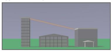
Two or more buildings are connected by CableFree wireless products. Clear Line-of-Sight (LOS) for FSO or Near-Line-of-Sight (NLOS) for radio is required.
